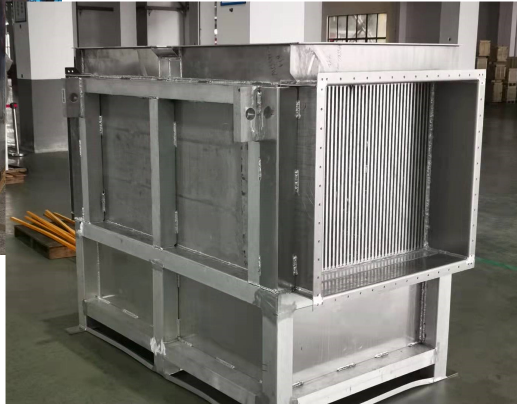
Heat exchanger for heat recovery system
